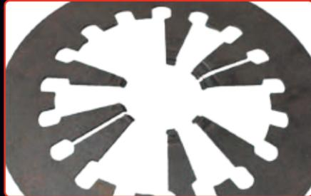
Misalignment between engine and transmission.
