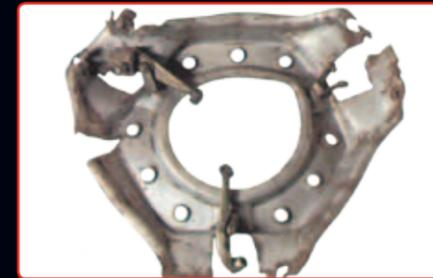
Centrifugal failure of 11 inch clutch due to non-standard installation. Possibly in lieu of twin plate.
