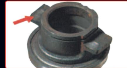
Worn release bearing carrier.
