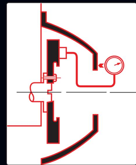
**STEP 2** With indicator still mounted to flywheel ensure rear surface of housing is square. SPECIFICATION: 0.15mm max. T.I.R.
