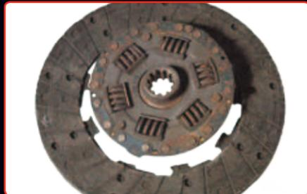
Clutch has failed at the segment necks due to misalignment between engine and transmission. Most common cause being non standard engine installation ie, engine transplant or engine not aligned with transmission first motion shaft.
