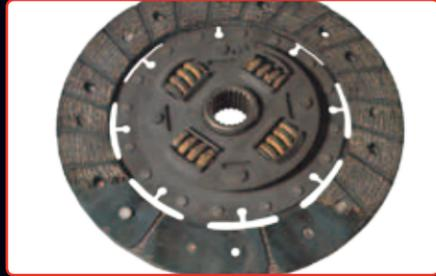
Burst facing usually caused by driver abuse, such as severe down changing through gears, ie 5th to 2nd at excessive road speed.
