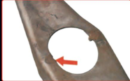
Unable to achieve clutch release. Failed release fork caused by incorrect release bearing carrier.
