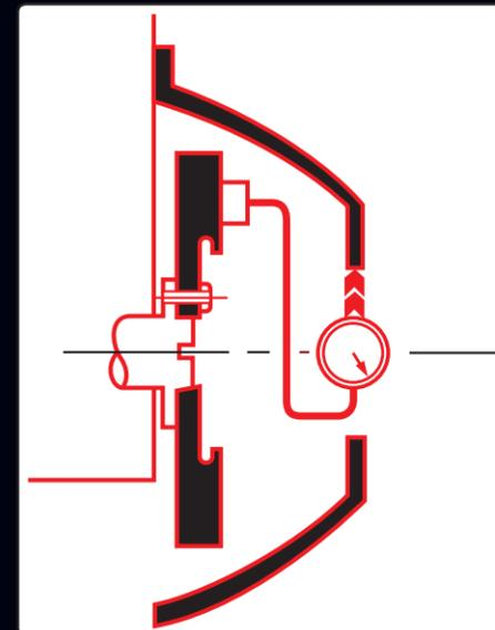
**STEP 1** Mount indicator to flywheel and determine concentricity of bell housing bore to centre line of crank rotation. SPECIFICATION: 0.15mm max. T.I.R.
