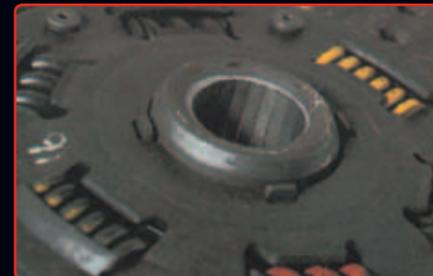
Result of incorrect clutch driven plate for the application.
