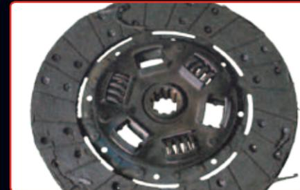
Incorrect cover assembly or incorrect clutch release mechanism adjustment or driver abuse.
