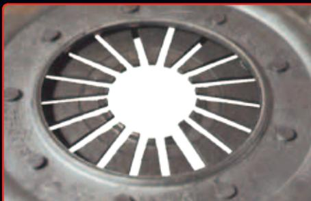
Clutch operation has deteriorated over a period of time. Misalignment has caused premature wear on pivot points within the cover assembly.
