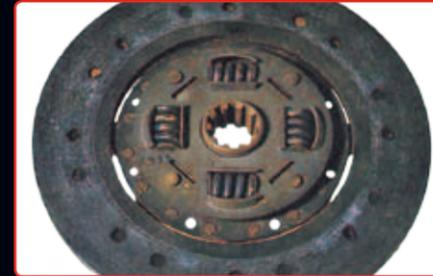
Heavy duty (wide facing) clutch plate installed under standard cover assembly (narrow pressure plate)
