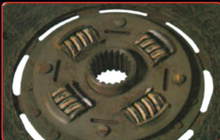
Clutch plate installed 'back to front'. Spring windows fouling the flywheel attaching bolts.
