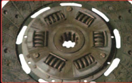
Contamination from faulty transmission seal or excessive lubrication of clutch release bearing.
