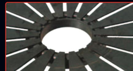
Misalignment between engine and transmission has resulted in the release bearing welding itself to the diaphragm.
