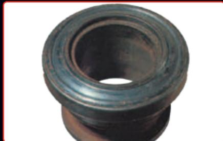
Incorrectly assembled release bearing (mounted 'back to front') on the carrier.
